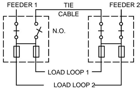
**Type 9 Pair** – Air Insulated Switchgear. Used to feed two loops or a large service. May be automated as a preferred/alternate scheme with the tie closed and an automatic transfer between the two feeders. Open points in the loops may exist at loadbreak elbows. The lack of a fuse in the tie allows the switchgear to make a live tie between two substations as it transfers load from one source to another.
