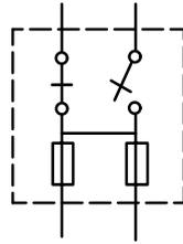
**Type 9** – Air Insulated Switchgear. Two switches and two fuses for loads. Used for loop end points with a companion Type 9 or Type 12 unit, or alone to feed very small loads where only one underground feeder exists.
