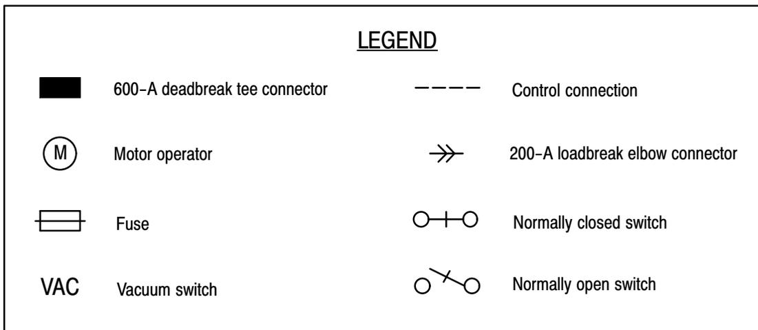
**Figure 1 – Automatic Retrofit Switchgear Schematic**
