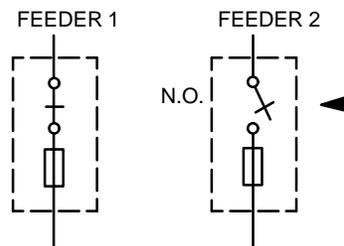
**Type 5 Pair** – Air Insulated Switchgear. For loop end points at the same location or for a complete dual primary service. May be automated to transfer automatically for loss of the normal source (see below).
