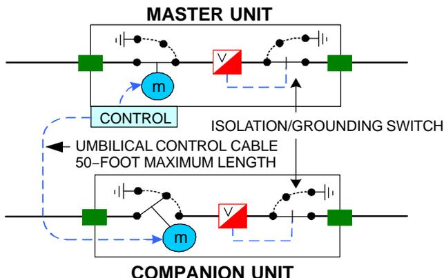
**Type 211 Automatic Pair** – SF6 Insulated Switchgear. Used for loop end points at the same location or a complete dual primary service. Automated (as shown above) to transfer for loss of the normal source.
