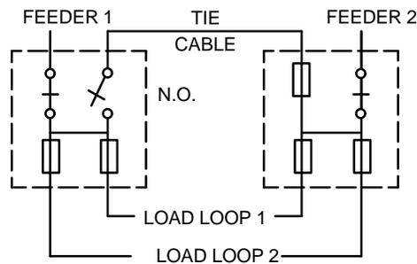
**Type 9/12 Pair** – Air Insulated Switchgear. Used to feed two loops or a large service. May be automated (see below) as a preferred/alternate scheme with the tie closed and an automatic transfer between the two feeders. Open points in the loops may exist at loadbreak elbows. The fuse in the tie prevents a unit fault from interrupting two feeders.
