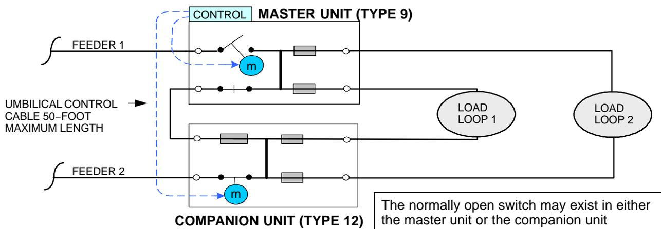
**Type 9/12 Automatic Pair** – Air Insulated Switchgear. Used to feed two loops (as shown above) or a large service. Automated as a preferred / alternates scheme with the tie closed and an automatic transfer between the two feeders. Open points in the loops may exist at loadbreak elbows. The fuse in the tie prevents a unit fault from interrupting two feeders.
