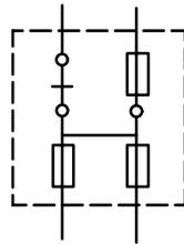
**Type 12** – Air Insulated Switchgear. One switch and three fuses. Used as a companion unit with a Type 9 where a protection point is needed in the tie between the two supply feeders to the switchgear installation. Never used alone.
