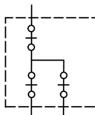
**Type 13** – Air Insulated Switchgear. Used to split very large loops into segments or to provide feeder sectionalizing.
