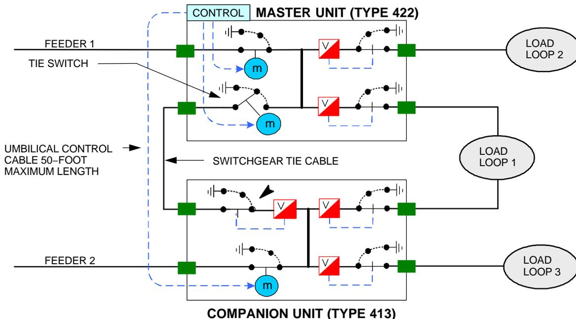
**Type 413/422 Automatic Pair** – SF6 Insulated Switchgear. Used for supply to two to four loops (more than two requires remote ends for the loops) or very large services. The automatic transfer mode may be preferred / alternate or main – tie – main depending on how the control is programmed. Only these automated versions are Standard.
