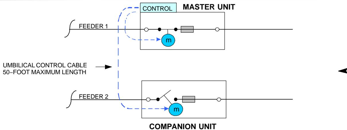
**Type 5 Automatic Pair** – Air Insulated Switchgear. For loop end points at same location or for a complete dual primary service.
